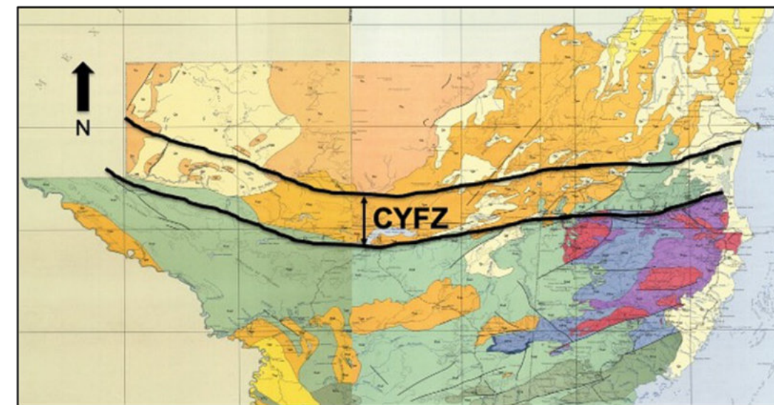
Figure 5. Geological map of Belize and northern Guatemala. The Central Yucatan Fault Zone (CYFZ) separates Paleozoic/Mesozoic rocks (blue, red and green) south of the fault zone from Tertiary rocks (earth tones) exposed within and north of the fault zone. Map from Bonis, Dengo and Bohnenberger, 1960.
