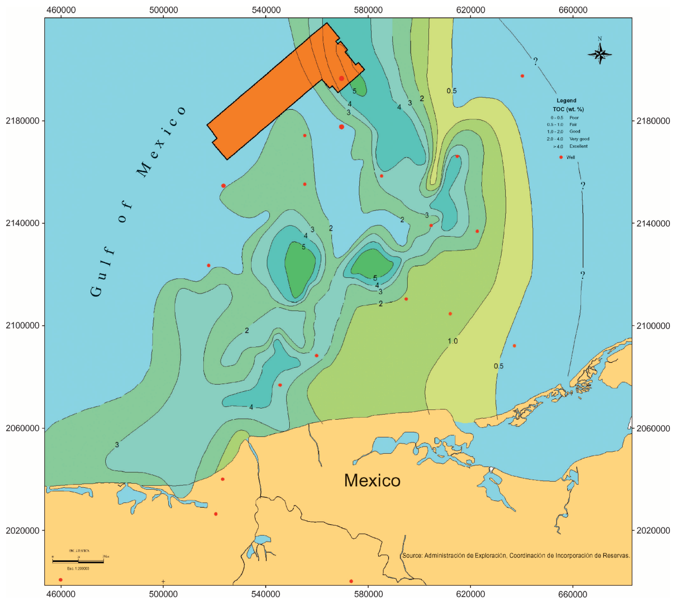
FIGURE 4. Map of Tithonian total organic carbon (TOC) distribution in the Campeche marine region and the study area. Source of data: Activo región Marina, PEMEX.
