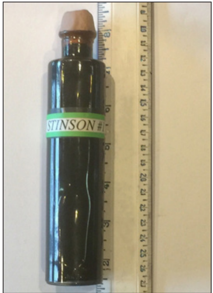
Figure 4. A. Probable Cambrian age orthoquartzite core from the Stinson #1 well showing highly fractured character and oil staining. B. Light brown oil (~37 API) from open-hole test at 14863'-15194' (corresponding to the top of the Cambrian orthoquartzite and basal few feet of the overlying Tertiary Canning Formation).
