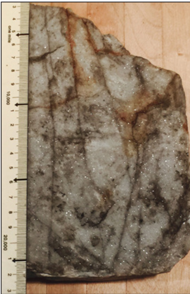
Figure 4. A. Probable Cambrian age orthoquartzite core from the Stinson #1 well showing highly fractured character and oil staining. B. Light brown oil (~37 API) from open-hole test at 14863'-15194' (corresponding to the top of the Cambrian orthoquartzite and basal few feet of the overlying Tertiary Canning Formation).
