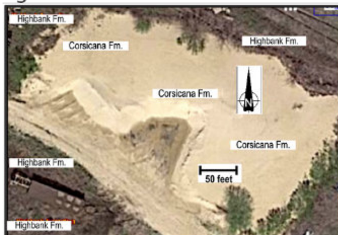
Figure 6B: Contact between Highbank and Corsicana formations at Texas Materials Clay Pit south of Austin along Colorado River. Excavation at clay pit created a man-made window revealing Corsicana Formation below Highbank Formation.
