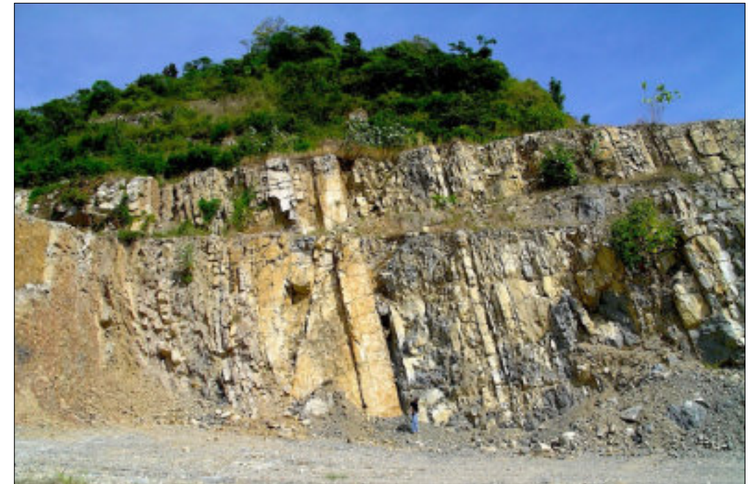
FIG 2. Steeply tilted and intensely fractured limestones—affected by both natural deformation and blasting—and gently folded strata of the Lower Apón Formation (Cogollo Group), exposed at the Catatumbo Quarry, Perijá Range, western Venezuela.
