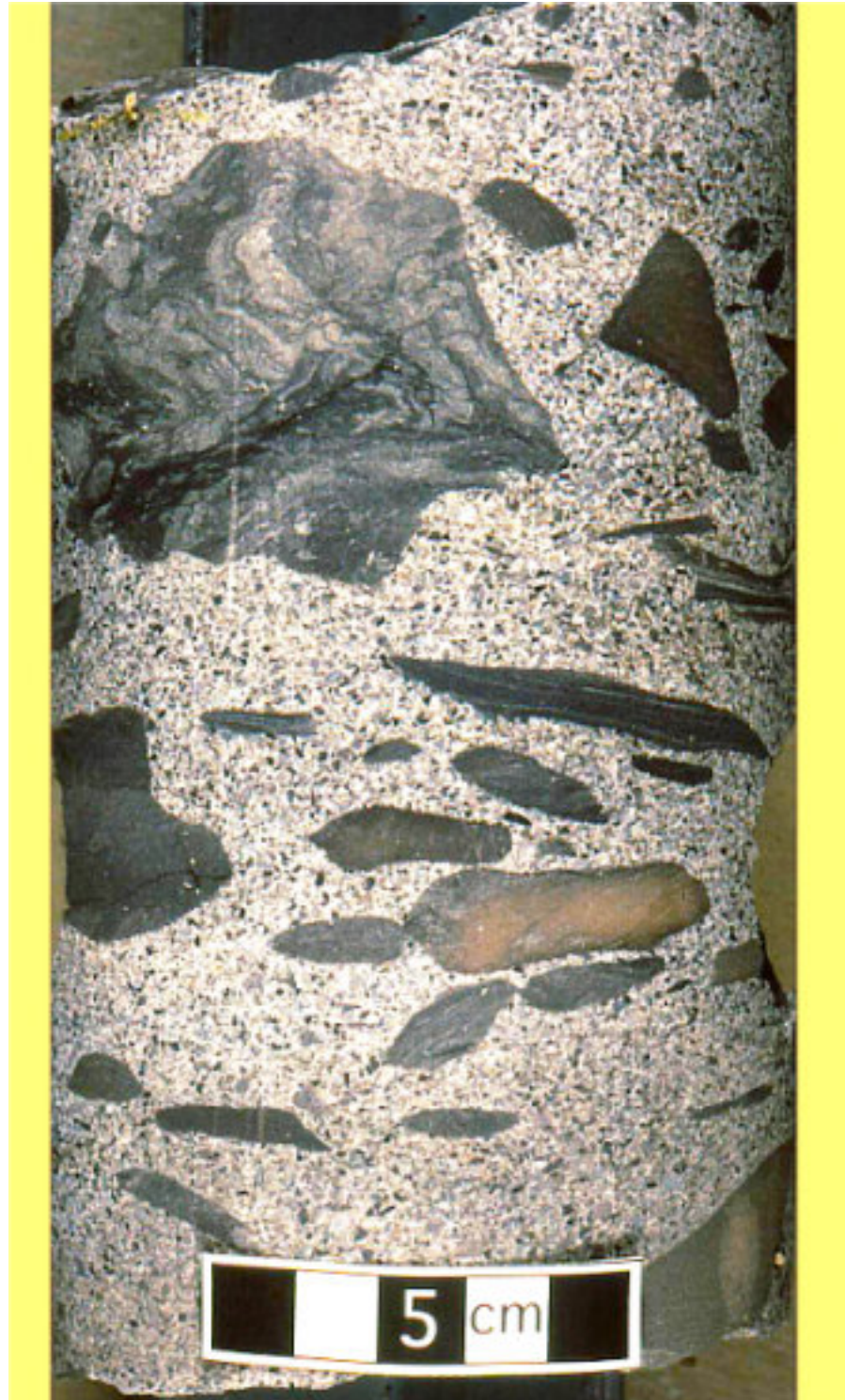
Fluvial channel basal lag, showing different mud clasts size and shapes. Core 6-17-72-9W6. Depth 1724.7 meters (Spirit River Formation – Falher D unit), Alberta, Canada. Photo by Jhonny E. Casas .
